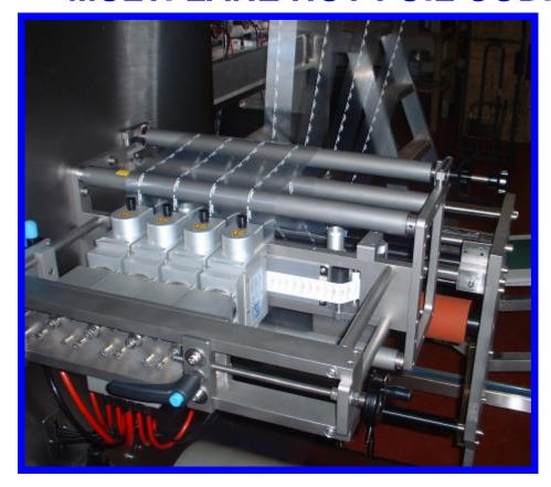
The Open Date ML Series is a self contained, multiple lane hot foil overprinting system. It provides an on-line contact overprinting solution where a single substrate has to be coded a number of times across it's width and where previously it has been necessary to fit complete hot foil printers for each lane.
