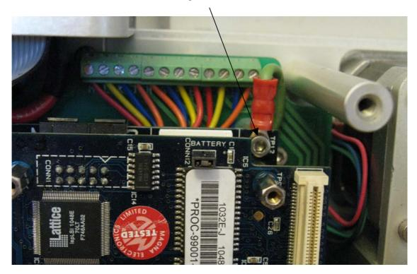
The battery type should be a 3Volt Lithium CR 2450N Coin Cell Battery
