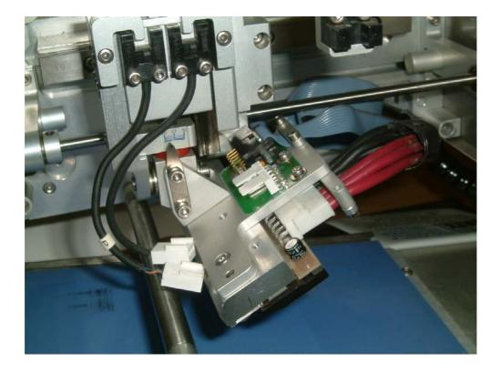
Remove the two fixing screws using a 2.5 Allen key
