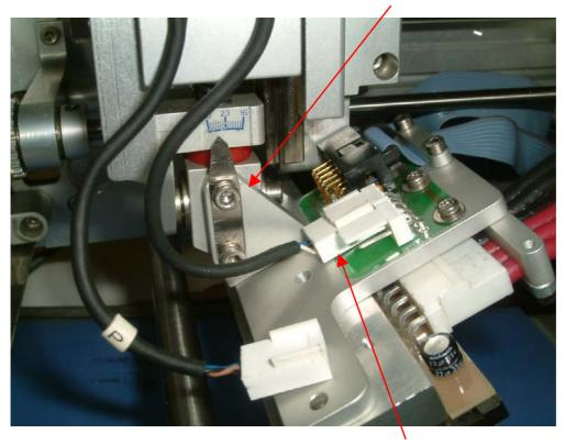
Set the Print head angle shown on the bottom of the head.
