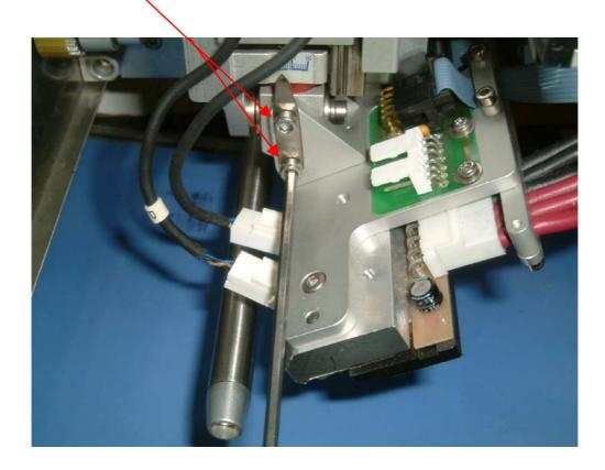
Remove the two retaining screws using a 2.0 Allen key holding the cable clamp. Then remove the ribbon cable.
