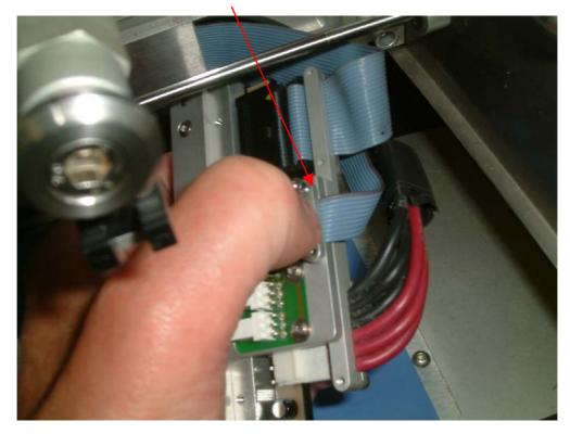
Take care not to pinch the ribbon cable in the retaining clamps
